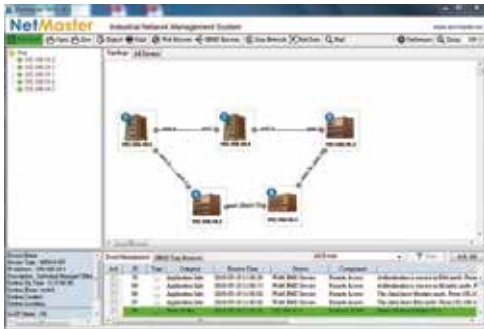
Automatic Discover and Intuitive Visualization of Network Devices and Topology
